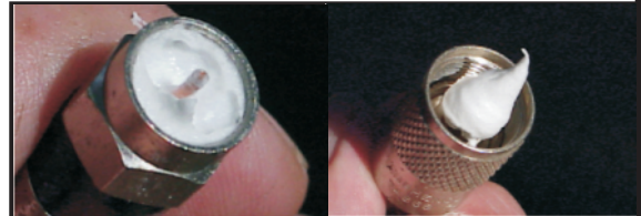
Correct STUF fill volume should be +/- Twice the estimated internal void volume when assembled.
