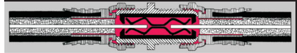
Cross Section of f-splice: RED indicates internal air voids filled with STUF
